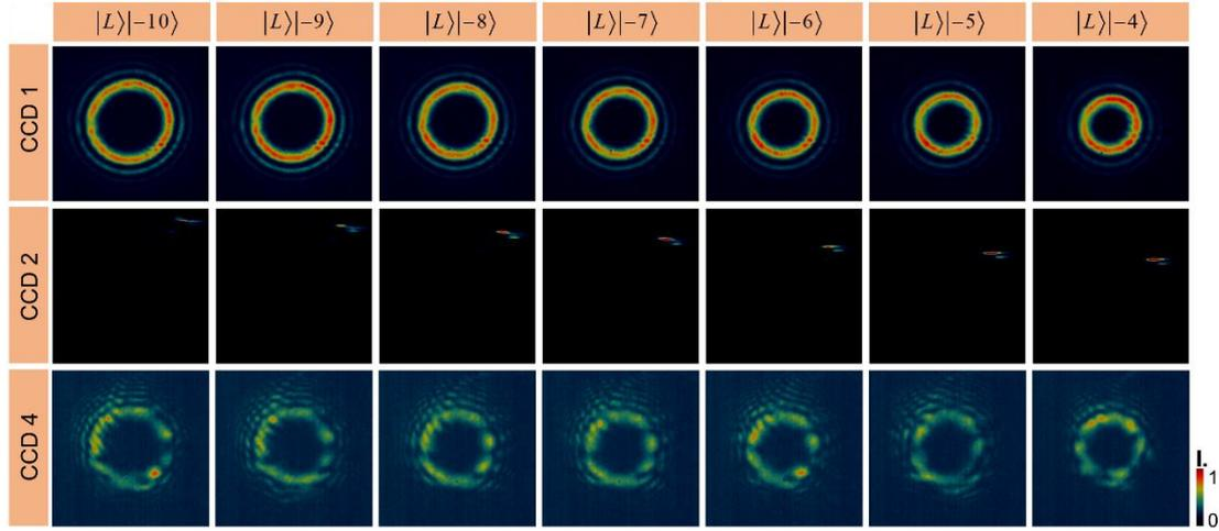
**Fig. S12** The experimental intensities distributions of single TAM states at CCD1, CCD2 and CCD4.  $|\psi\rangle = |L\rangle|l\rangle$ ,  $l = -10 \sim -4$ .
