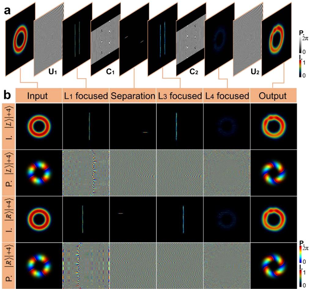
**Fig. S3 Transformation process of TAM manipulator for TAM mode  $|\psi\rangle = (|L\rangle + |R\rangle)|+4\rangle$ .** (a) the propagation detail where  $L_1 \sim L_4$  are omitted. (b) intensities and phases distributions of various observing planes of two single TAM components  $|L\rangle|+4\rangle$  and  $|R\rangle|+4\rangle$ .
