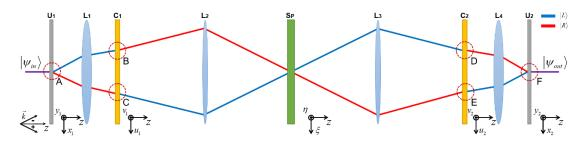
**Fig. S2 Principles of TAM mode recovers through the proposed TAM reverser.** U<sub>1</sub>, unwrapper; L<sub>1~4</sub>, lenses; C<sub>1</sub>, corrector; S<sub>P</sub>, separation (filter) plane; C<sub>2</sub>, anti-corrector; U<sub>2</sub>, anti-unwrapper.
