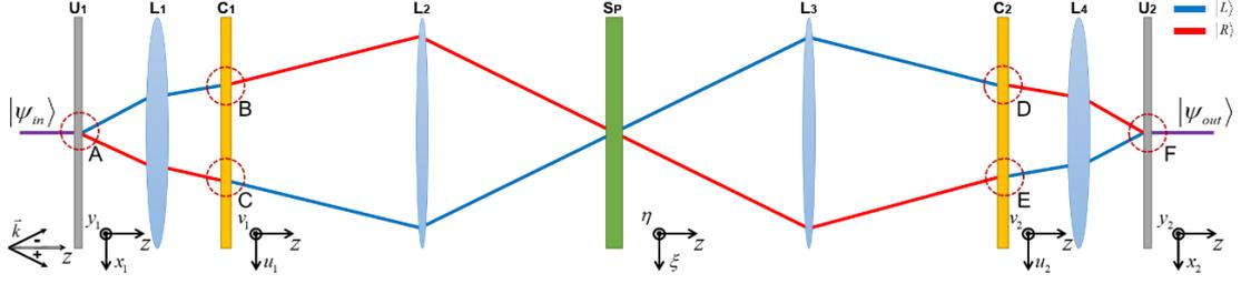
**Fig. S2 Principles of TAM mode recovers through the proposed TAM reverser.**  $U_1$ , unwrapper;  $L_{1-4}$ , lenses;  $C_1$ , corrector;  $Sp$ , separation (filter) plane;  $C_2$ , anti-corrector;  $U_2$ , anti-unwrapper.
