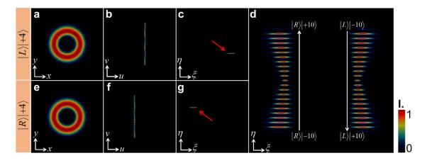
Fig. S1 Simulated intensities distributions of single TAM states on input plane (a) (e), rear focal plane of lens  $L_1$  (b) (f), and separation plane (c) (g). Simulated intensities distribution of all 42 single TAM states in separation plane (d).
