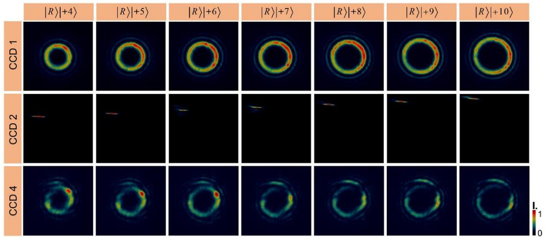
**Fig. S17** The experimental intensities distributions of single TAM states at CCD1, CCD2 and CCD4.  $|\psi\rangle = |R\rangle|l\rangle$ ,  $l = +4 \sim +10$ .
