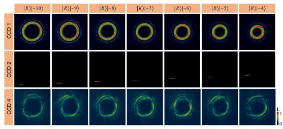
Fig. S15 The experimental intensities distributions of single TAM states at CCD1, CCD2 and CCD4.  $|\psi\rangle = |R\rangle |l\rangle$ ,  $l = -10 \sim -4$ .
