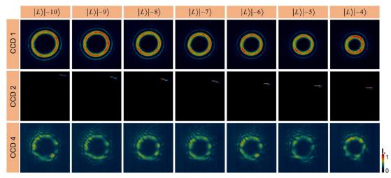
Fig. S12 The experimental intensities distributions of single TAM states at CCD1, CCD2 and CCD4.  $|\psi\rangle = |L\rangle|l\rangle$ ,  $l = -10 \sim -4$ .
