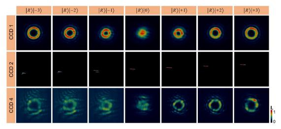
Fig. S16 The experimental intensities distributions of single TAM states at CCD1, CCD2 and CCD4.  $|\psi\rangle = |R\rangle |l\rangle$ ,  $l = -3 \sim +3$ .
