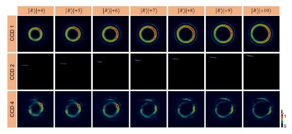
Fig. S17 The experimental intensities distributions of single TAM states at CCD1, CCD2 and CCD4.  $|\psi\rangle = |R\rangle|l\rangle$ ,  $l = +4 \sim +10$ .
