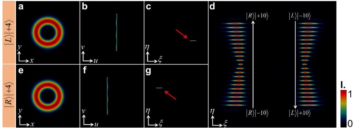
**Fig. S1** Simulated intensities distributions of single TAM states on input plane **(a)** **(e)**, rear focal plane of lens  $L_1$  **(b)** **(f)**, and separation plane **(c)** **(g)**. Simulated intensities distribution of all 42 single TAM states in separation plane **(d)**.
