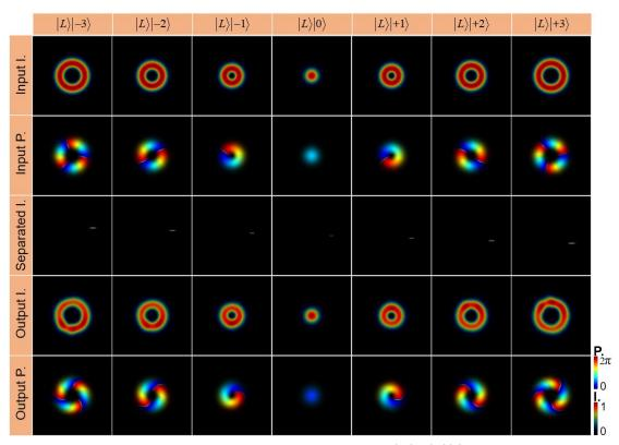
Fig. S7 The simulated results of single TAM states.  $|\psi\rangle = |L\rangle|l\rangle$ ,  $l = -3 \sim +3$ .
