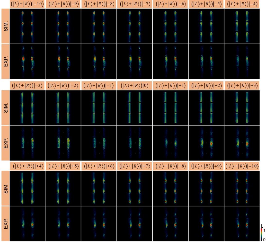
**Fig. S19** The simulated and experimental patterns of linear polarized OAM beam at the rear focal plane of the lens  $L_1$ .  $|\psi\rangle = (|L\rangle + |R\rangle)|l\rangle$ ,  $l = -10 \sim +10$ .
