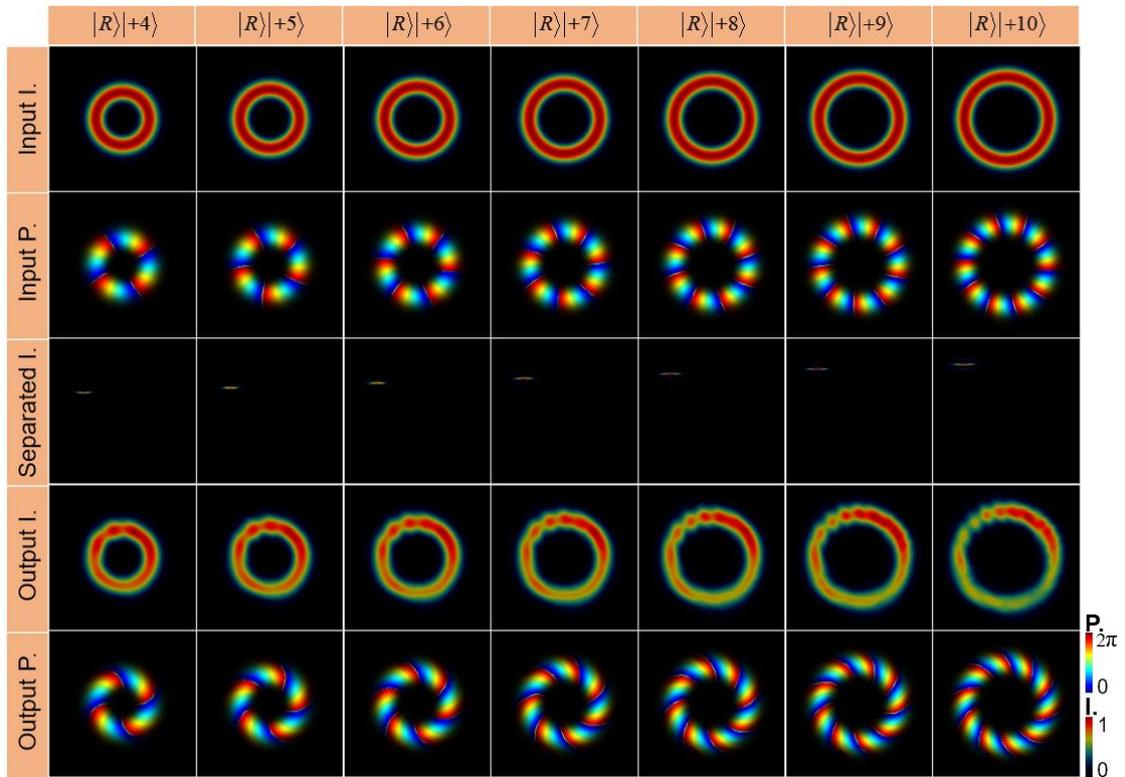
Fig. S11 The simulated results of single TAM states.  $|\psi\rangle = |R\rangle|l\rangle$ ,  $l = +3 \sim +10$ .
